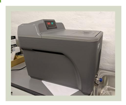
System for cleaning of supporting materials of 3D prints using dissolving solution and heat. The device is essential since the support material is difficult to remove, especially in the case of small details.
