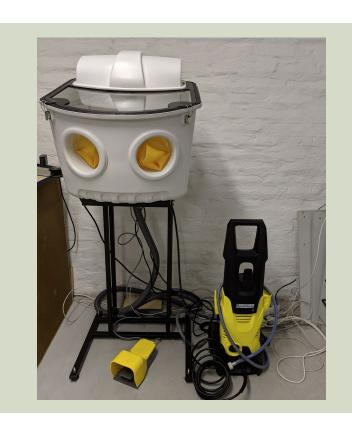
System for the rinsing of supporting materials of 3D prints. The device is essential since the support material is difficult to remove, especially in the case of small details.
