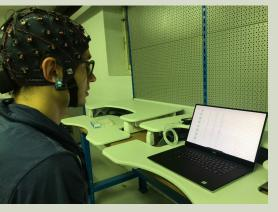
EEG system for testing the response of users while using computer systems, for research in the field of brain-computer interaction and similar research. 64-channel EEG system from g.tec enables precise measurements of electric potentials on the skull and, thus, study of mental processes. Enables integration into extended system for tracking users at interaction with devices.
