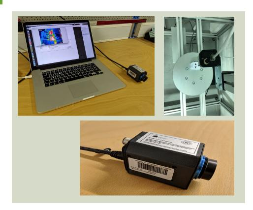
Thermal camera for sensing temperature of objects. Suitable for acquisition of thermal images of people/faces that can provide information related to physical and psychological conditions.
