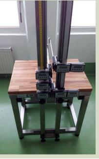
• A stadiometer is used to measure the spinal curves (lumbar, chest and neck). It can evaluate the change in spinal curves over a certain period (e.g., before and after an 8-hour sitting and before and after an 8-hour sitting with active breaks). The stadiometer is extremely accurate since it allows reading the measurements to three decimals
