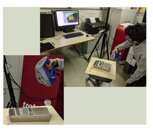
Handheld 3D scanner with metrological accuracy. The scanner is capable of high resolution 3D scanns and can capture 3D point clouds and textures. It is an essential tool for reverse engineering and digitalisation of 3D objects that can be used in immersive digital environments. The scanner also comes with high performance software Artec Studio.
