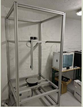
Working table for prototype setups of computer vision systems. Includes a rotational and linear drive that enables controlled image acquisition of objects from different angles and distances.
