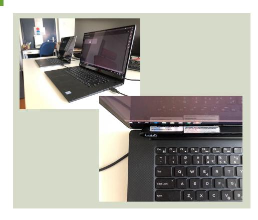
System for gaze tracking for simultaneous testing of large user groups while they are using user interfaces and testing user experience, and to observe the behavior of different user groups (including, for example, users with special needs, illnesses, etc.) when using computer systems. The special feature of this system is that it allows operation on larger screens and contains an API key that allows full access to the source data. Owner institution:
