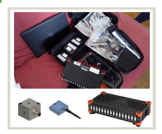
For monitoring and assessment of building and building component vibrations with calculation of periods, mode shapes, etc.:
