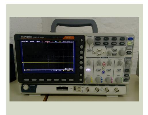
Laboratory instrument used to display and analyze the waveform of electronic signals.
