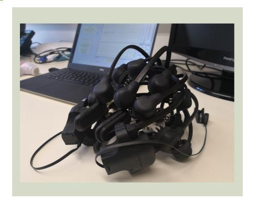
20 channel wireless **EEG headset** with dry electrodes. Enables quick setup and mobility due to Bluetooth connection. The software supports LabStreamLayer to connect to other software for data analysis.
