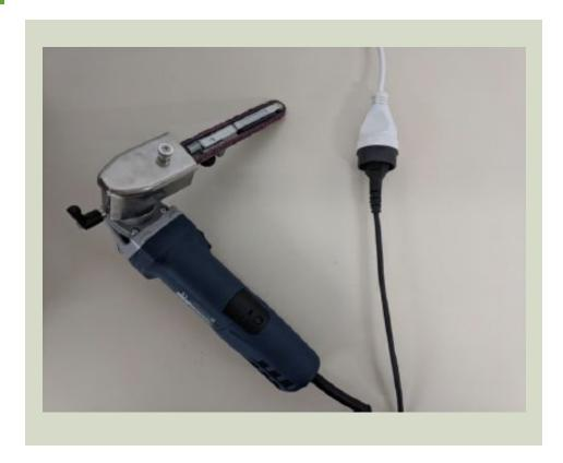
File for shaping and grinding precise things.
