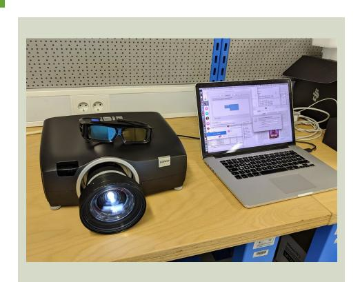
A high frequency refreshment projector that can project onto moving objects for research in the field of ambient augmented reality where any object can become an interactive display.
