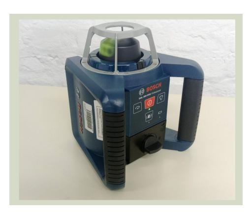
Control tool consisting of a laser beam projector useful for setting up virtual reality frames to which various sensors are attached or for installing wall interactive elements.
