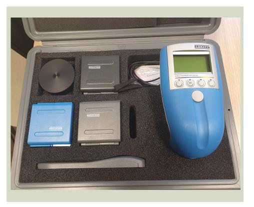
The spectrometer is a mobile device used to quantify color and gloss of objects.
