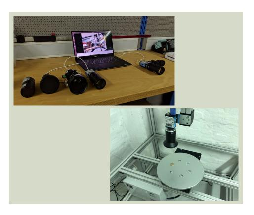
A system of two industrial USB 3.1 12MP cameras with lenses f=8, 12 (2x), 25 (2x), 35 and 50mm. For development of computer vision systems.
