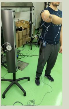
• The system enables precise and high frequency digital recording of reference points (markers) in 3D space. Markers are usually placed in pre-defined places on the human body, which are then recorded by the camera and converted into digital form. This allows accurate tracking of the observed motion in the room and further basic and advanced kinematic processing.
