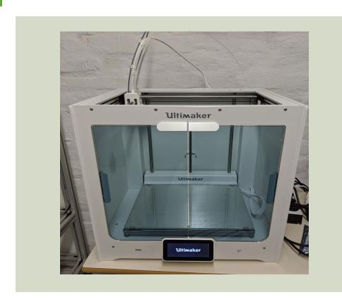
Desktop 3D printer with FDM technology that allows 3D printing of simple objects. Its specialty is the extremely low price of basic material and maintenance of the device.
