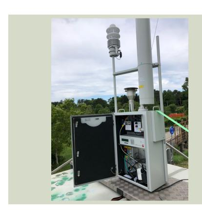
The Model 365 is a mobile stand-alone environmental monitoring station that is used for monitor air pollution.
