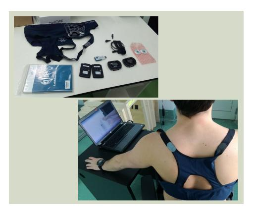
Sensor, mounted on human body that measures ECG, heart rate, breathing rate, skin temperature, activity and body position and connects to external sensors for data storage and transmission. It is used in sports, ergonomics and rehabilitation research.
