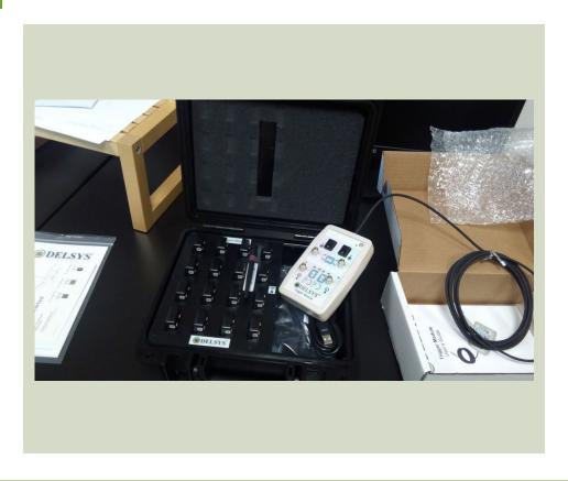
The electromyography measuring system is aimed at implementing the electromyography method. Electromyography is a noninvasive electro-diagnostic method for assessing and recording electrical activity caused by skeletal muscles. The measuring system enables the simultaneous evaluation of muscular activity on 16 different muscles.
