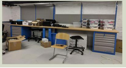
A set of work desks for various jobs (soldering, cutting, grinding, etc.) with drawers for storing tools, meters, oscilloscopes and other building materials.
