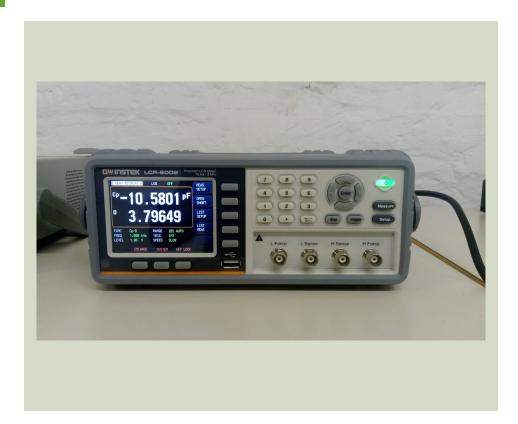
LCR meter is a type of electronic test equipment used to measure the inductance (L), capacitance (C), and resistance (R) of an electronic component.
