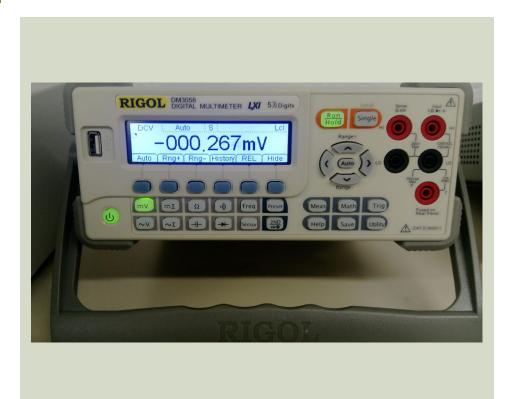
Multimeter, multitester or a VOM (volt-ohm-milliammeter) is an electronic measuring instrument for measuring voltage, current and resistance.
