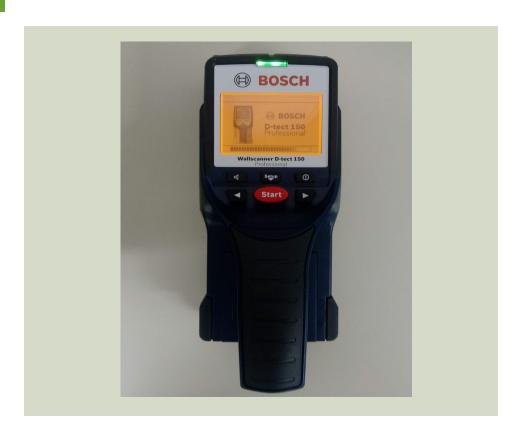
A device for locating various materials in the walls and ceilings required when mounting wall or ceiling interactive devices or frames supporting such devices.
