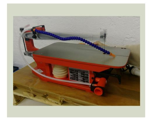
Precise modelling saw for cutting precise pieces of plastic or wood to produce supporting elements of interaction devices.
