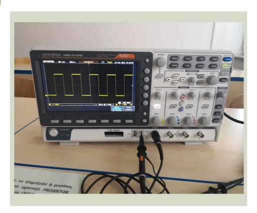
100Mhz 4-channel analog and 16-channel digital inputs. Enables spectral analysis, signal decoding and analysis for I2C/SPI/UART/CAN/LIN, signal filtering functions.
