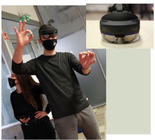
Hololens2 is a mixed reality head-mounted display that can be used for generating immersive augmented reality experiences. The device is fully mobile with advanced ondevice processing capabilities.
