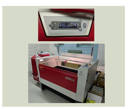
Laser cutter for the manufacture, processing and cutting of pieces for various housings and pieces of computer-aided devices or stands (for example, a wooden head mount display case) and for supporting various research tasks.
