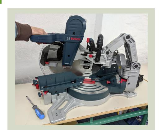
A saw used to make accurate crosscuts and miters in a workpiece and cuts of different angles for preparing samples and prepare raw elements for fabrication.
