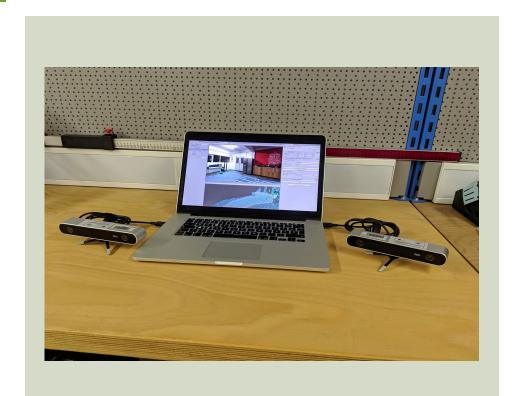
Stereoscopic camera for 3D reconstructions, capturing structures from motions or 3D scanning. The camera is used to create computer interfaces through computer vision and for the purpose of 3D reconstruction.
