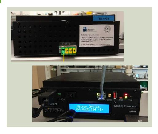
The si155 is an industrial grade fanless optical sensing interrogator. Featuring both static and dynamic full spectrum analysis, the si155 provides long-term, reliable and accurate measurements of hundreds of sensors on 4 parallel, 160 nm wide channels.
