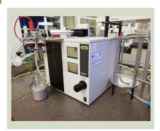
Device disintegrates extrudable solutions into equally-sized droplets, followed by chemical or physical solidification. Beads are produced with single nozzle system (150 µm to 2000 µm), while concentric nozzles fabricate core-shell morphology (400 µm to 1800 µm in diameter).
