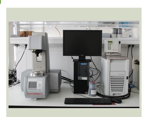
Enables performance of rheology tests on a variety of materials in rotational and oscillatory mode using different measuring systems: cone-plate, plate-plate and concentric cylinders. Measuring system allows simulation of coating processes, polymer/gel cross-linking, etc.
