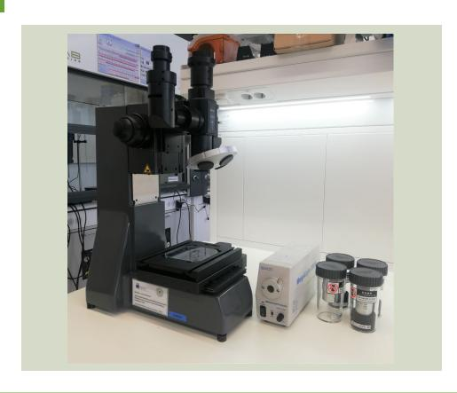
Modular miscroscope unit with open configuration for integration of lasers with a wide applicable wavelength region: near-infrared-visible-near-ultraviolet radiation. Equipped with a set of apochromatic objective lenses (magnifications: 10X, 20X, 50X, 100X) which enable large working distances.
