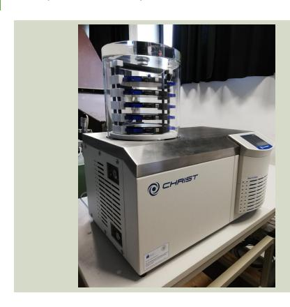
Freezeing solidifies samples and shapes their morphology; freeze drying removes frozen water through sublimation, preventing pore collapse and resulting in porous structures. Ice condenser can reach down to - 90° C, while T-programmable shelves and temperature sensors enable a multiphase design of the drying process and its control.
