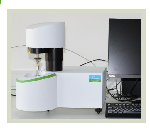
The TGA instrument enables reproducible determination of temperature decomposition and studies of material combustibility, sample volatility, moisture and solvent content, and oxidation stability. Measurements can be performed in the temperature range from -15° C to 1200° C.
