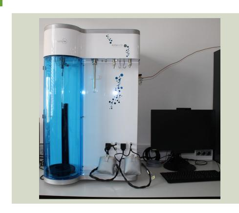
Determination of the specific surface area, size and distribution of meso- and micro-pores of materials of different shapes in the pore diameter range from 0.5 to 500 nm via adsorption of gas molecules. The apparatus consists of three separate analysis stations which allow simultaneous analysis of three powder samples.
