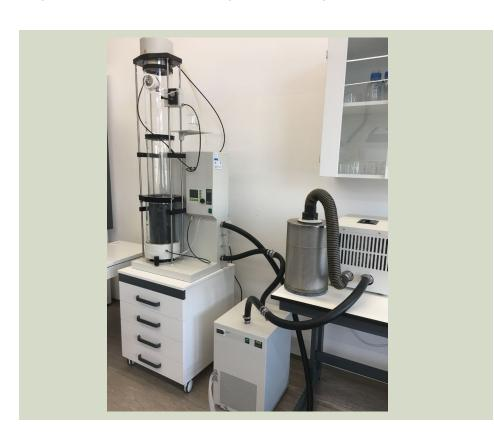
Water-based samples (i.e. solutions, nanoemulsions and nanosuspensions) are atomized into fine droplets and dried in a flow of drying gas, resulting particles, ranging from 200 nm to 5 µm. Atomization takes place in nebulizers inside spraying head, droplets are dried within the drying chamber and particles are captured by the collecting electrode and deposited on the wall of the collecting cylinder.
