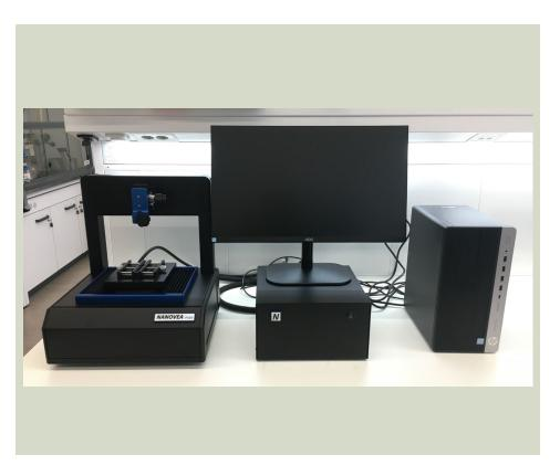
Optical profilometer for morphology analysis of flat samples of varying degrees of roughness, e.g. thin polymer films, polymer coatings on different substrates, porous membranes and electrospun fibrous mats. Measurements are performed in a non-contact mode using continuous scanning with no need for stitching and an ability to perform measurements on tilted, curved samples with varying degree of reflectivity.
