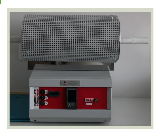
Single zone tube furnace with a maximum heating temperature of 1200° C with integrated ceramic work tube and an additional work tube made of impermeable aluminum ceramics for processes in inert atmosphere. The pyrolysis furnace enables calcination of inorganic particles and carbonation of polymeric materials.
