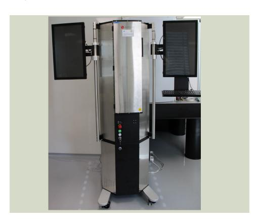
The welder is based on welding technology with the implementation of a CO2 laser. A special technology called Axicon Splicing allows the user to "design" a laser beam i.e. changes the area and radius of the active zone and laser output. The latter enables welding of special optical fibers of different dimensions, producing long and even tapering of the fiber structures (so-called "tapering") and production of other special photonic structures.
