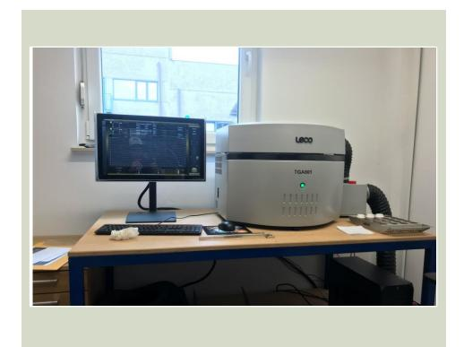
Moisture, Ash, Volatile Content, And Loss-On-Ignition
