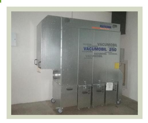
Vacuum system for aspiration of dust produced during woodworking operations, equipped with frequency inverter, pressure control unit and fire extinguisher
