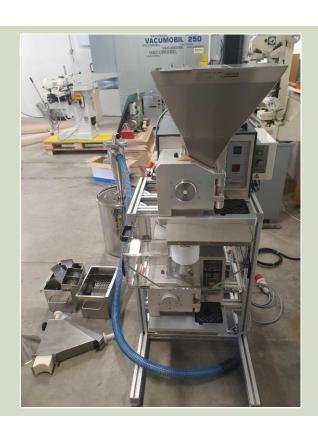
Grinder is equipped with two grinding stations for continues and batch grinding
