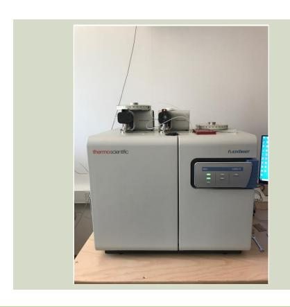
Carbon, hydrogen, nitrogen, sulfur and oxygen (CHNS/O) analyses.
