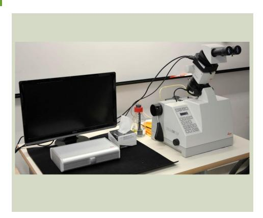
Mechanical surface preparation device for microscopy. Uses grinding, cutting, and polishing fixtures to prepare mirror like surfaces of a variety of materials.
