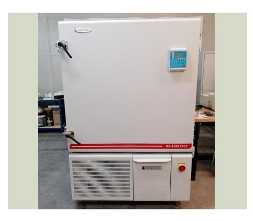
1000l volume climatic chamber operating in the range -40° C to 180° C, and relative humidity range: 10-98%. Suitable for material temperature & RH resistance and product testing, sample conditioning, accelerated ageing and stress tests.
