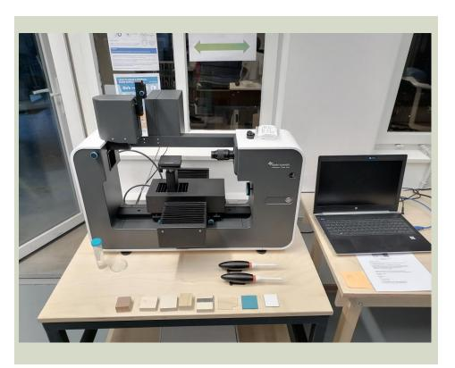
Designed for reliable and repeatable measurements of wettability and adhesion. Possibility to measure: static and dynamic contact angle, roll-off angle, surface free energy, surface tension, interfacial tension, batch contact angle and roughness corrected contact angle.
