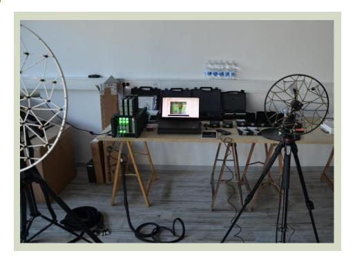
The acoustic camera enables sound source localization and sound intensity measurements using acoustic holography and beamforming.
