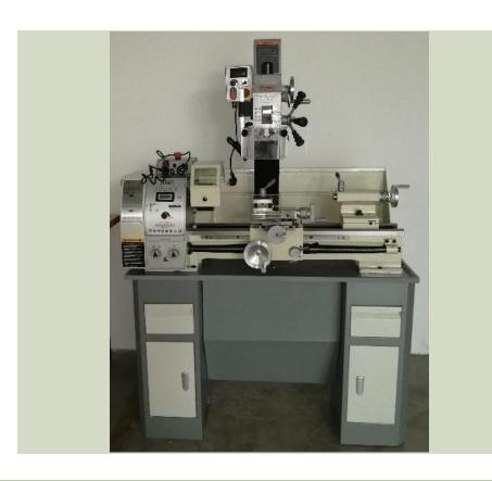
Metal working machine for turning, milling and drilling operations performed on the metal parts used in prototypes
