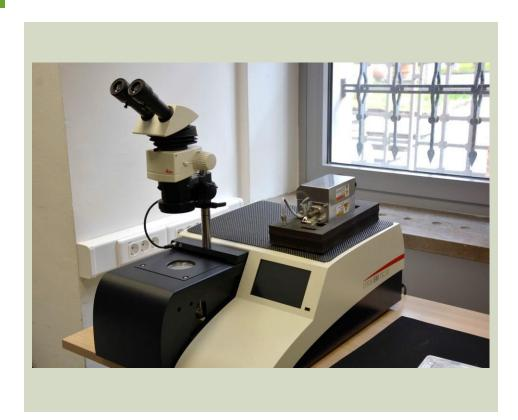
Creates near-perfect surfaces of materials for microscopy using accelerated argon ions. Capable of cross-cuts (4 mm x 1 mm) and surface milling of 25 mm<sup>2</sup> areas. Includes a cooling stage for heat sensitive materials.
