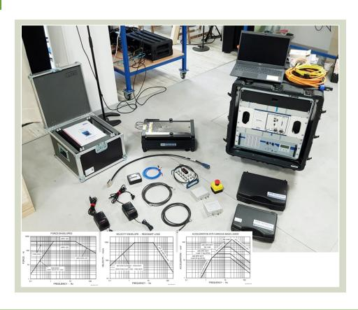
Portable shaker, (with accessories) for dynamic excitation of structures:
