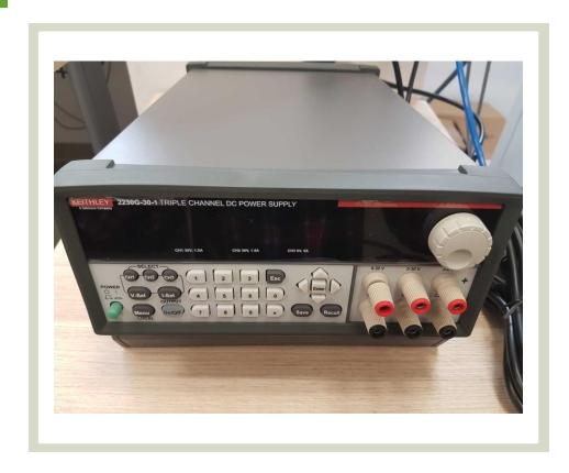
High Power, 3-Channel Programmable Power Supplies. Complete control of the power supplies from a PC; LabView and IVI drivers facilitate instrument control, data logging, and analysis..
