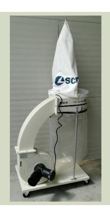
Vacuum system for aspiration of dust produced during woodworking operations
