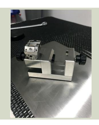
Sample holder with wider ange rotation for solid sample surface preparation
