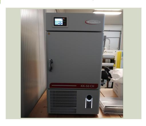
50l volume climatic chamber operating in the range + 5° C to 180° C, and relative humidity range: 10-98%. Suitable for material temperature & RH resistance and product testing, sample conditioning, accelerated ageing and stress tests.
