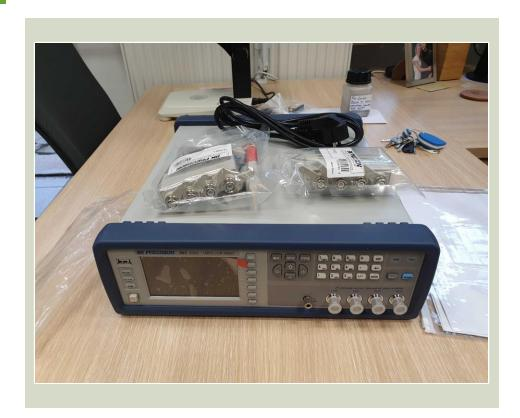
LCR meters capable of measuring inductance, capacitance, and resistance of components and materials at DC
