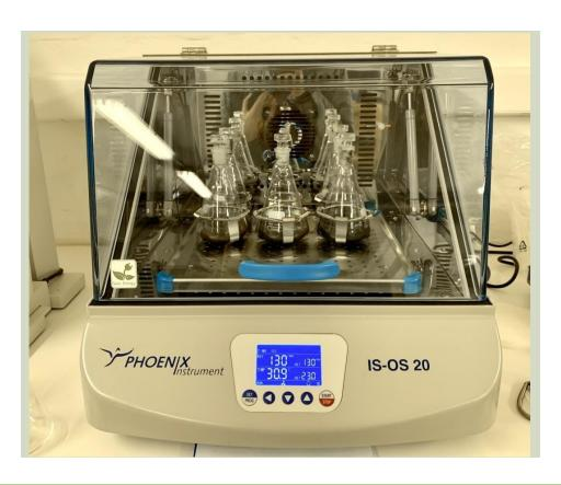
Temperature controlled (+5 - 60 C)20mm amplitude
