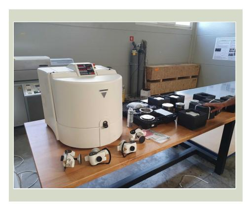
For fine wet and dry grinding for mixing and homogenizing of emulsions and pastes and dry materials using four working stations.
