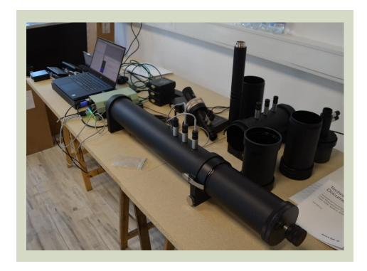
Using tubes of different diameters measurements are performed in the 50 Hz to 6 kHz frequency range.
