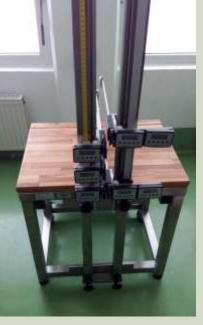
• A stadiometer is used to measure the spinal curves (lumbar, chest and neck). It can evaluate the change in spinal curves over a certain period (e.g., before and after an 8-hour sitting and before and after an 8-hour sitting with active breaks). The stadiometer is extremely accurate since it allows reading the measurements to three decimals.
