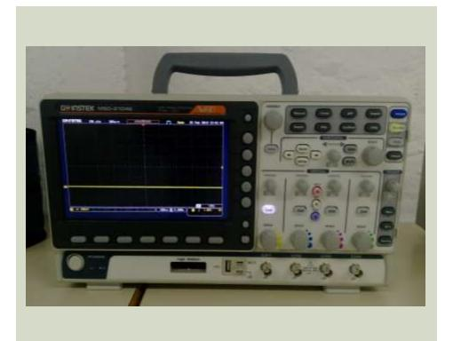
Laboratory instrument used to display and analyze the waveform of electronic signals.
