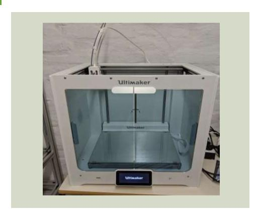
Desktop 3D printer with FDM technology that allows 3D printing of simple objects. Its specialty is the extremely low price of
