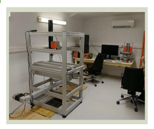
Five hyperspectral cameras covering following the bands: VNIR (400-1000nm), NIR (900-1700nm), SWIR (1000-2500nm), MWIR (2.7-5.3μm) and LWIR (8-12.4μm)) produced by SPECIM and two dedicated scanners (20cm x 40cm and 50cm x 100cm) allow chemical mapping of various materials. The software can be used for exploratory, qualitative and quantitative analysis.
