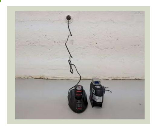
Control tool consisting of a laser beam projector useful for setting up virtual reality frames to which various sensors are attached or for installing wall interactive elements.
