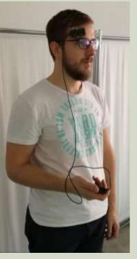
Near-infrared-spectroscopy (NIRS) is a spectroscopic method that uses the near-infrared field of the electromagnetic spectrum (from 780 nm to 2500 nm). This method is used in medical, sports, ergonomic and rehabilitation research.
