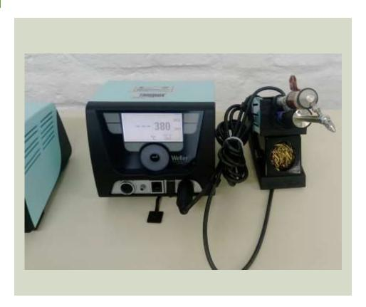
Device designed for de-soldering electronic components used in electronics and electrical engineering.
