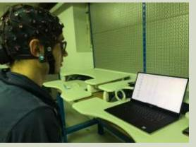
EEG system for testing the response of users while using computer systems, for research in the field of brain-computer interaction and similar research.
