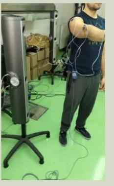
The system enables precise and high frequency digital recording of reference points (markers) in 3D space. Markers are usually placed in pre-defined places on the human body, which are then recorded by the camera and converted into digital form. This allows accurate tracking of the observed motion in the room and further basic and advanced kinematic processing.
