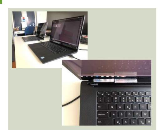
System for gaze tracking for simultaneous testing of large user groups while they are using user interfaces and testing user experience, and to observe the behavior of different user groups (including, for example, users with special needs, illnesses, etc.) when using computer systems. The special feature of this system is that it allows operation on larger screens and contains an API key that allows full access to the source data.
