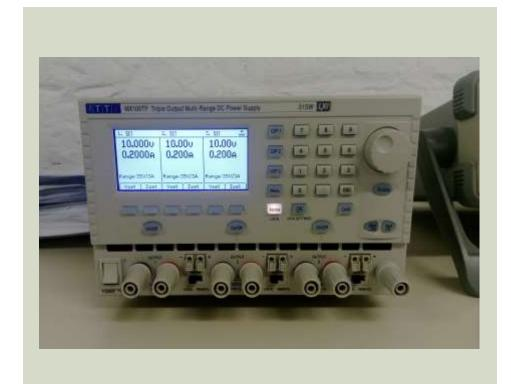
Electrical device that supplies electric power to an electrical load by converting electric current from a source to the correct voltage, current, and frequency to power the load.
