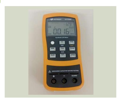
Portable electronic test equipment used to measure the inductance, capacitance, and resistance of an electronic component.
