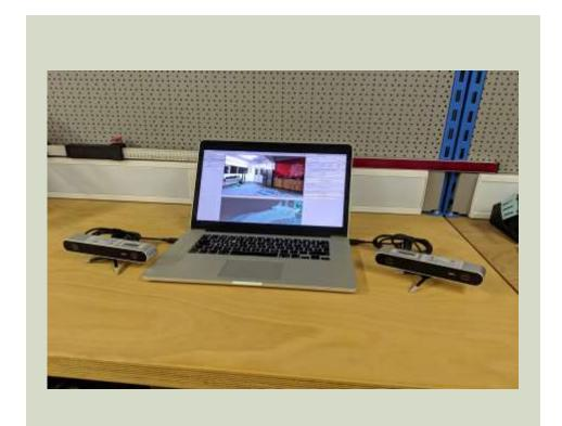
Stereoscopic camera for 3D reconstructions, capturing structures from motions or 3D scanning. The camera is used to create computer interfaces through computer vision and for the purpose of 3D reconstruction.
