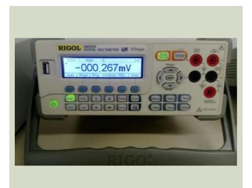
Multimeter, multitester or a VOM (volt-ohm-milliammeter) is an electronic measuring instrument for measuring voltage, current and resistance.
