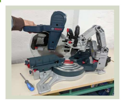
A saw used to make accurate crosscuts and miters in a workpiece and cuts of different angles for preparing samples and prepare raw elements for fabrication.
