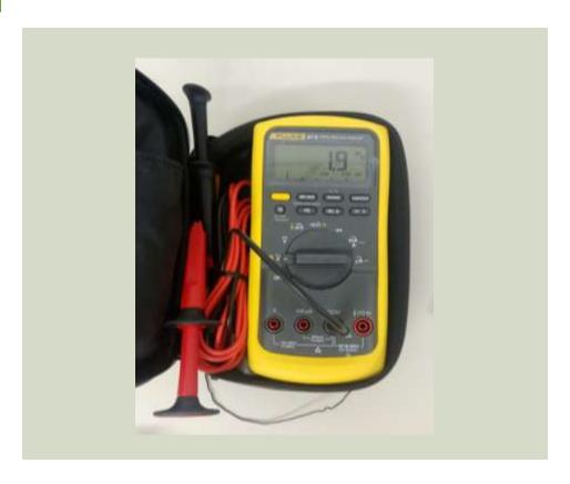
Portable electronic measuring instrument for measuring voltage, current, and resistance.
