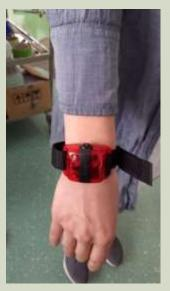
Accelerometer ActiGraph is designed to evaluate the intensity of movement activity. With the help of the accompanying software, it gives us the information about time we spent in low, moderate and high activity. It also gives us the information on the number of steps and energy consumption. In addition, we can evaluate the quality of sleep.
