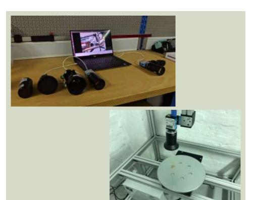
A system of two industrial USB 3.1 12MP cameras with lenses f=8, 12 (2x), 25 (2x), 35 and 50mm. For development of computer vision systems.
