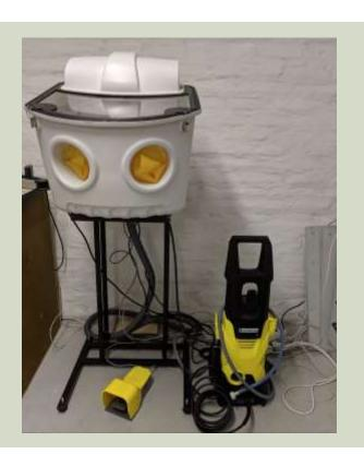
System for the rinsing of supporting materials of 3D prints. The device is essential since the support material is difficult to remove, especially in the case of small details.
