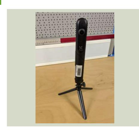
Camera to capture 360 degree video and stereoscopic video, which is then used in virtual worlds for various purposes, such as studying the immersiveness of such worlds, studying through experiential learning, etc.
