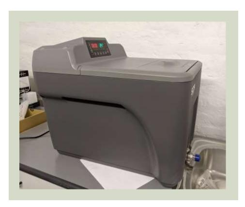
System for cleaning of supporting materials of 3D prints using dissolving solution and heat. The device is essential since the support material is difficult to remove, especially in the case of small details.
