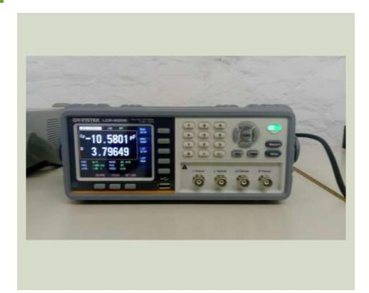
LCR meter is a type of electronic test equipment used to measure the inductance (L), capacitance (C), and resistance (R) of an electronic component.
