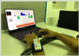
EMG & ECG system for studies in which we want to test the biological response of users in the use of computer systems for measuring arousal, immersiveness and other parameters.
