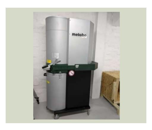
Waste extraction system from various machine tools. This machine is vital to lower the amount of dust in the lab.
