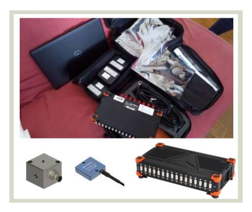
For monitoring and assessment of building and building component vibrations with calculation of periods, mode shapes, etc.:
