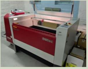
Laser cutter for the manufacture, processing and cutting of pieces for various housings and pieces of computer-aided devices or stands (for example, a wooden head mount display case) and for supporting various research tasks.
