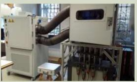
10 kN capacity long-term testing device. Five independent loading stations with fixtures for tension, three-point bending, and compression. Features a programmable environmental chamber for temperature and humidity control.
