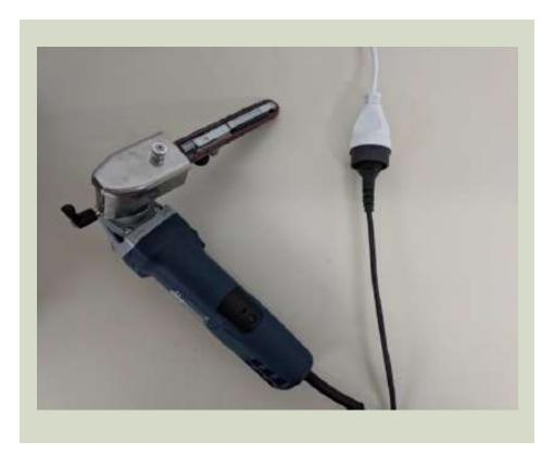
File for shaping and grinding precise things.
