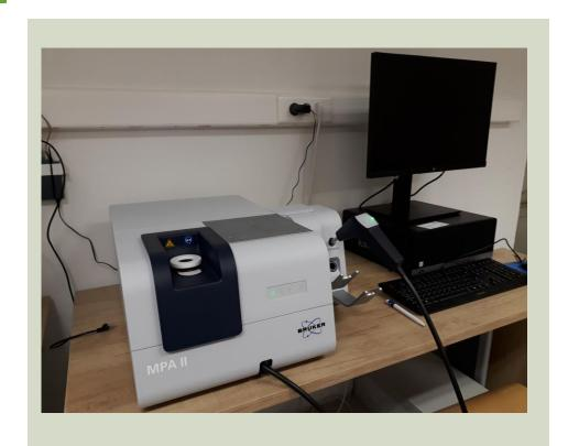
A fast and precise tool for the non-destructive analysis of liquid, solid and semi-solid materials. Equipped with fibre optic, integration sphere and transmission sample compartment for vials, operates in the range 11500-4000cm<sup>-1</sup>. The OPUS software allows data acquisition, processing, and evaluation.
