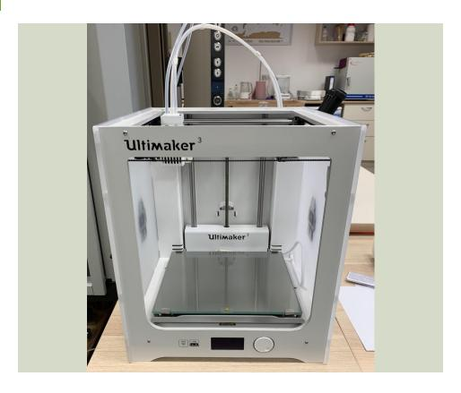
215 x 215 x 200 mm print size20 micron layer depthNozzle temperature up to 280 C
