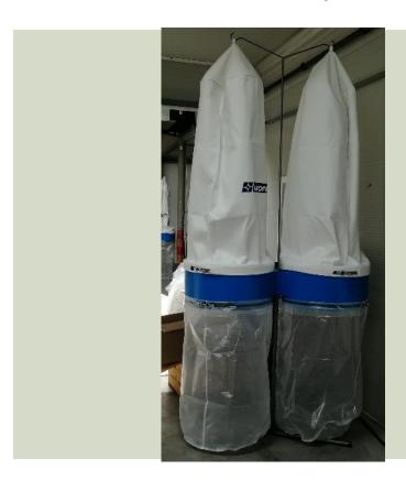
Vacuum system for aspiration of dust produced during woodworking operations
