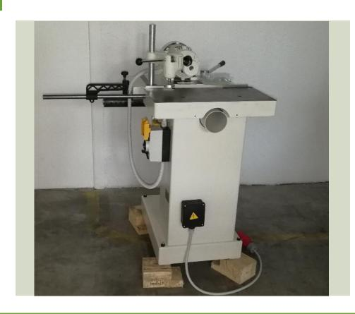
Wood working machine suitable for complex sample preparation and experimentations regarding machinability of materials and process/surface quality
