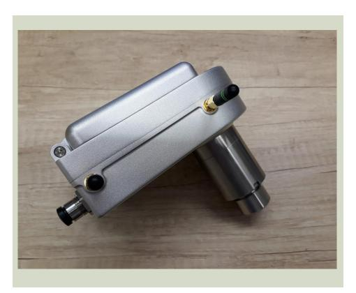
A system for real-time process monitoring in PAT applications. It has no moving components enabling superior instrument stability and performance in harsh process environments (IP67 standards). The system includes the VIAVI MicroNIR Pro software.
