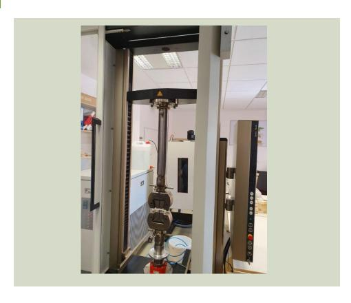
100 kN capacity universal testing machine. Includes fixtures for 3-point and 4-point bending, shear block, tension, and compression tests. Features a programmable environmental chamber for temperature and humidity control during testing; -40C to 200C and 10% to 85% RH
