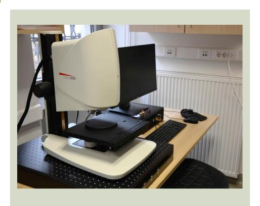
Combines multi-spectral imaging and confocal microscopy to image and measure material surfaces, map topography, and analyse surface roughness. Fully digital microscope with objectives from 1.25X to 150X.
