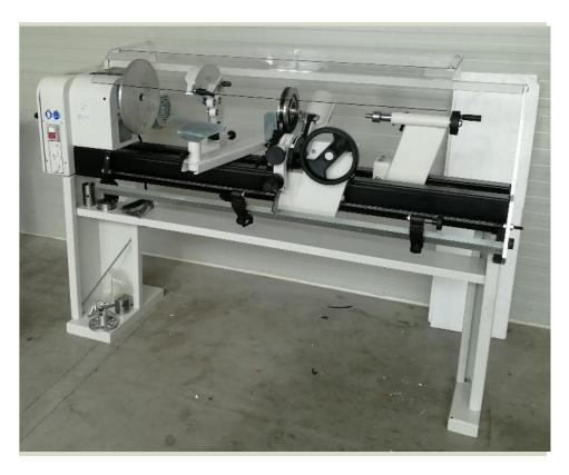
Wood working machine suitable for complex sample preparation and experimentations regarding machinability of materials and process/surface quality
