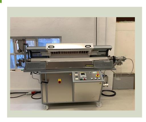
Equipped with gas system to incorporate CO2 and N2. Capable of batch and continuous processing with adjustable speed and tilting.
