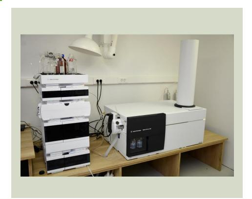
Used for the detection of biochemical and organic compounds in complex samples of environmental and biological origin. The double mass spectrometry detectors (quadrupole and TOF) allow to gain more structural information on your analyte based on the fragmentation pattern.
