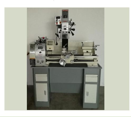
Metal working machine for turning, milling and drilling operations performed on the metal parts used in prototypes
