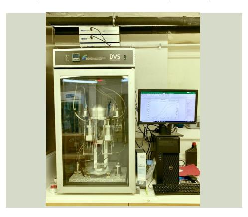
The DVS is used for measuring the sorption properties of materials.
