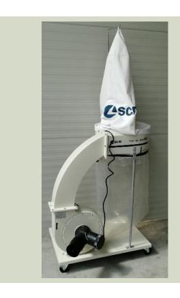
Vacuum system for aspiration of dust produced during woodworking operations
