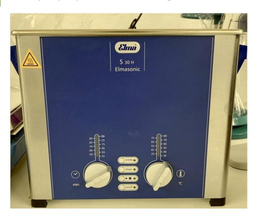
Used to clean samples or small laboratory equipment
