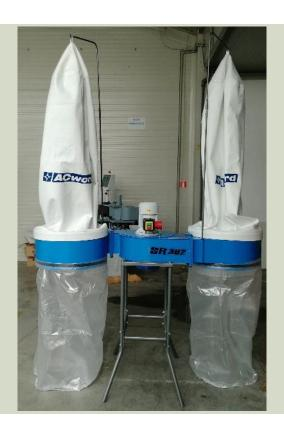
Vacuum system for aspiration of dust produced during woodworking operations
