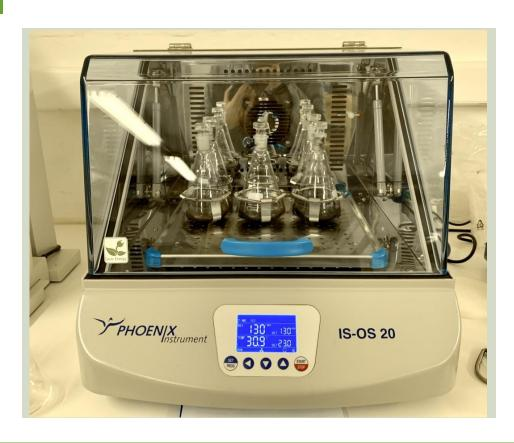
Temperature controlled (+5 - 60 C)20mm amplitude
