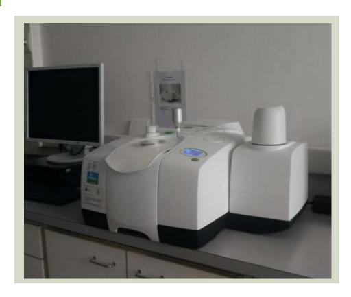
For infrared analysis of sample identity, composition, quality, and consistency.
