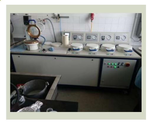
RK lab sheet former with equalizer is basic equipment in every papermaking laboratory. It is equipped with 4 vacuum driers and white water circulation system. Suitable to make sheets from different fibres, wood, and alternative biomass sources as well as glass wool, synthetic fibres, etc.
