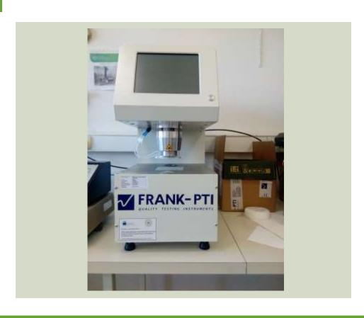
All-in-one Bendtsen tester to determine air permeability and roughness in mL/min and Gurley permeability in s. Measuring range is from 0 to 5000 mL/min. All measured data are recorded and statistically processed.
