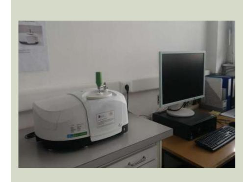
For infrared analysis of sample identity, composition, quality, and consistency. Standard optical system with KBr windows for data collection over a spectral range of 8300 – 350 cm<sup>-1</sup>.
