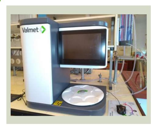
The analyser is capable to determine a wide range of fibre characteristics: length (0,01-7,60 mm), width (0,001 – 1 mm), fine particles, coarseness, curl, HW/SW ratio, fibrillation, kink index, cell wall thickness, etc.
