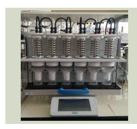
The automated extractor provides reliable and accurate results using an improved extraction Randall technique that is five times faster compared to the traditional Soxhlet method. The determination of extractable matter is performed with a solid-liquid extraction process that removes soluble components from solids using a liquid solvent.
