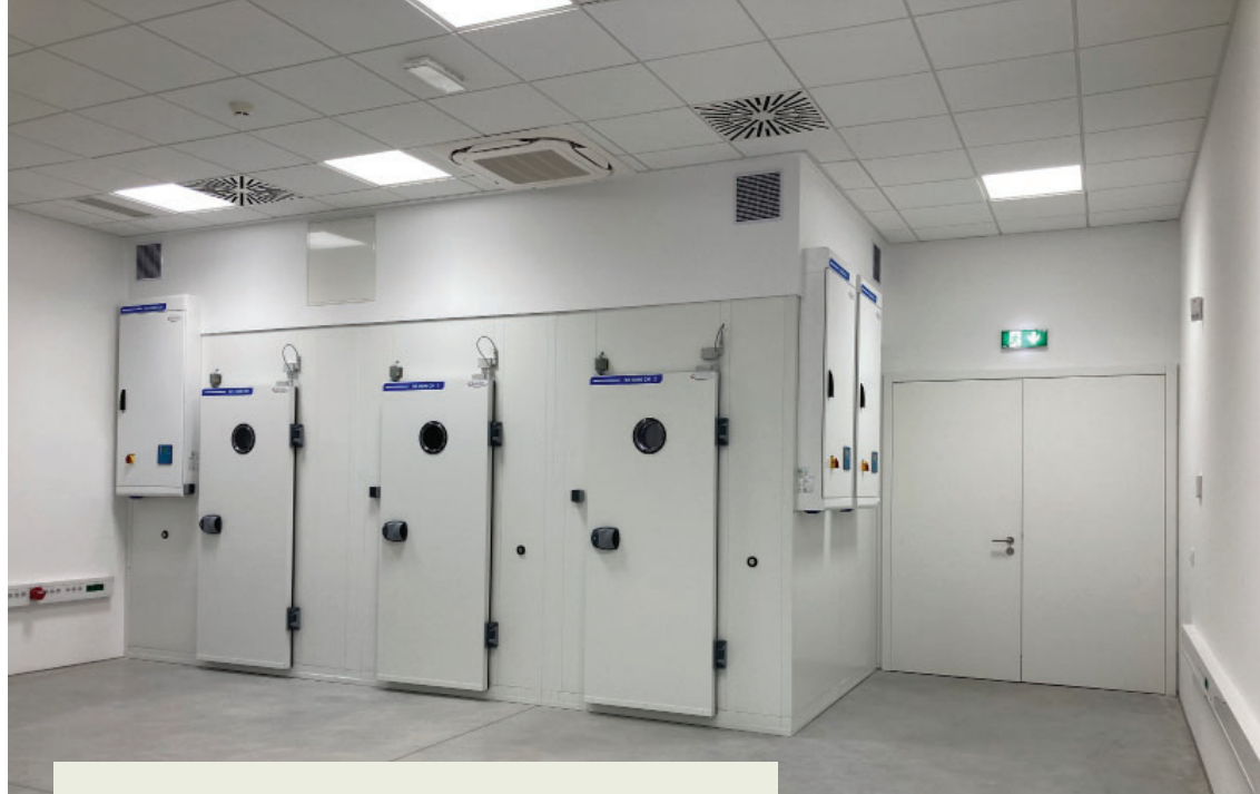
Climatic chamber in the Physical Testing Laboratory / Klima komore v laboratoriju za fizikalna testiranja
